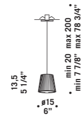
LUMÈ SF LUMÈ SFWD 1x46W E14 HSGSP/C/UB alogeno chiara clear halogen foro incasso \varnothing 4,5 cm recessed hole \varnothing 4,5 cm 1 x E14 LED LED light bulb
